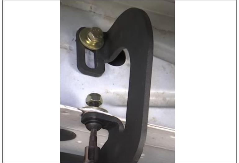
Step 12. Use (#9) M8 hex bolt, (#10) flat washer and (#11) lock nut to fasten the step to the bottom portion of (#5) and (#6) brackets.
