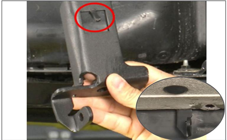
**Step 8.** Next, install (#6) second bracket using the supplied (#9) M8 hex bolt, (#10) M8 washer and (#13) M8 lock washer and leave loose for now.
