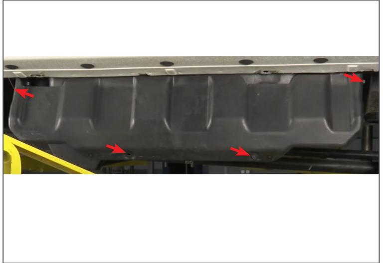
**Step 7.** Install (#5) first bracket by sliding up and behind the def tank until the upper tab locks into place in the body of the vehicle. Tug down firmly on the bracket until it hangs on its own and the welded nut it aligned with the hole in the pinch weld. This step may take a couple of tries.
